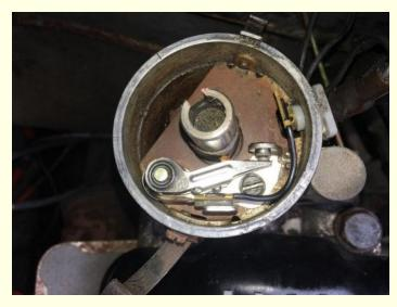
Coils can sometimes fail, but make no mistake about it - suspect the points first.
